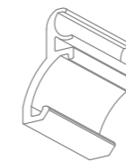
COVER HINGE to hold cover plate, installed on either side
